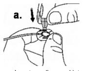
Insert needle guard into connector part.
