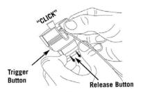
4. Pull back the release button until it clicks into place in activated position.
