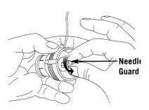
5. Twist to remove needle guard and retain for later use.
