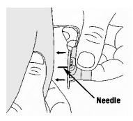
4. Pinch skin and insert the Quickset at a 90 degree angle.Smooth down the adhesive.
