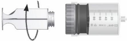
Twist the plastic pusher to remove it from the syringe assembly.
