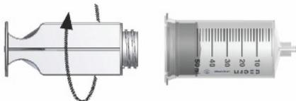
Twist the plastic pusher to remove it from the syringe assembly.
